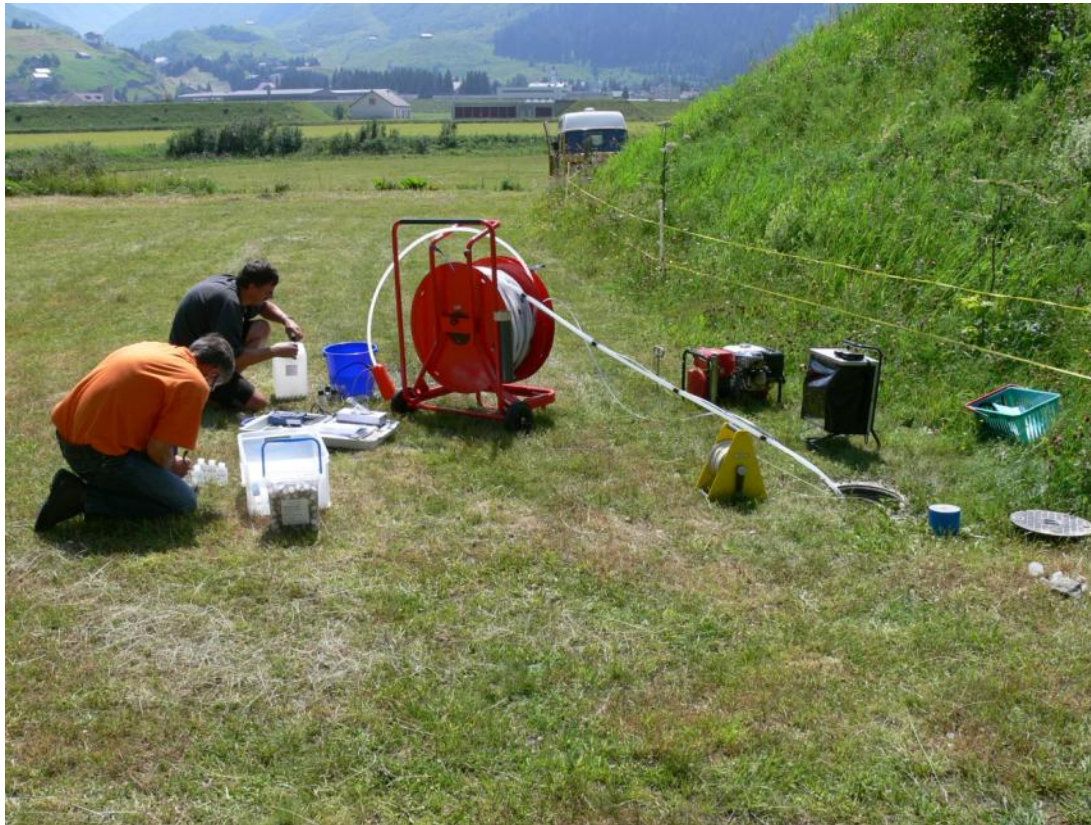
Figure 4: Groundwater sampling with the help of a groundwater pump from a borehole next to the backstop.
